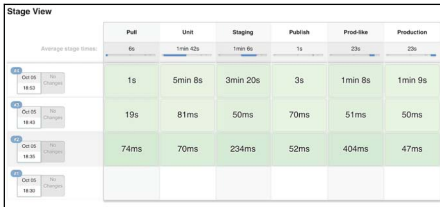
Figure 6-11: The Jenkins Pipeline Stage View screen
